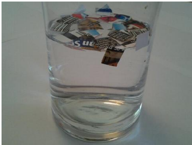
Roll on labels float in water
